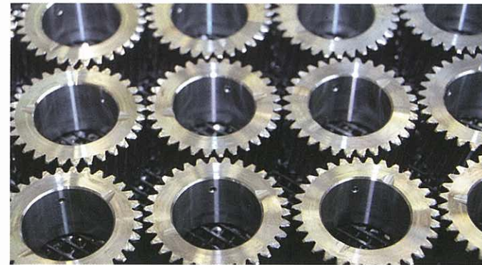
The planetary gears are manufactured in manageable lot sizes.
