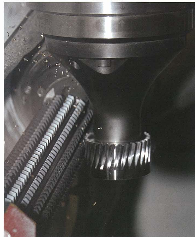
Gear cutting in progress at Voith's Garching facility.
